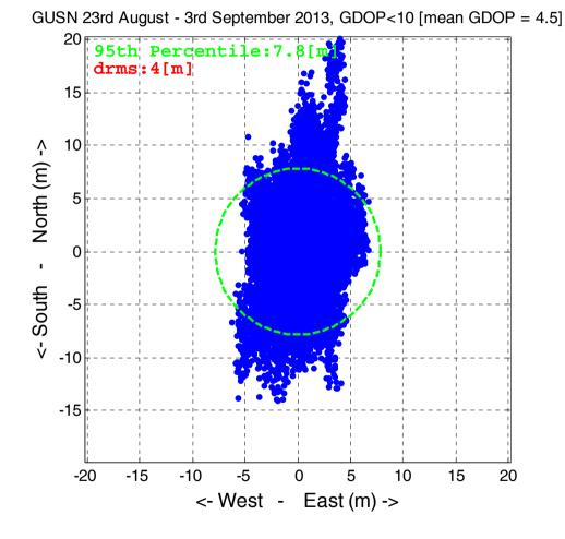
Dual Frequency Positioning Accuracy (PDOP <=5):
