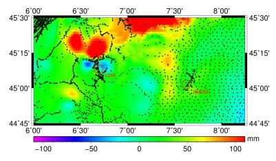
Figure : Differences between the new (EGG2015) and old (EGG2008) quasigeoid heights around INRIM and LSM (▲: new ITOC points; •: old points)
