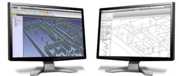
Walls and windows are automatically extracted and exported directly to Revit as the correct family objects.
