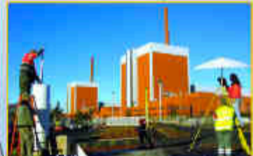
Critical site monitoring \Delta position \sim 0.1 mm/yr
