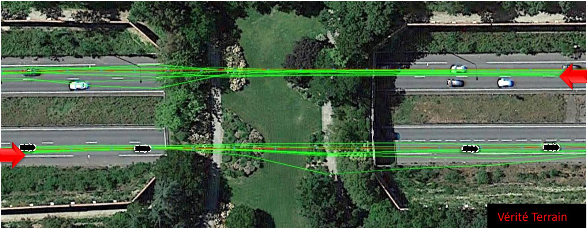
NB.: The trajectories are calculated by the same series of receivers on board a same vehicle
