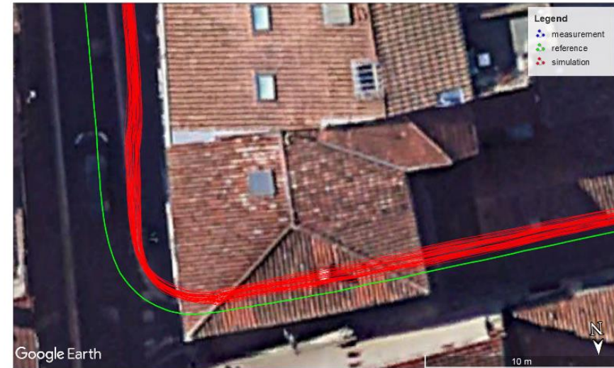
Figure A.3 – Simulated trajectories showing a turning within the urban environment long uniform street
