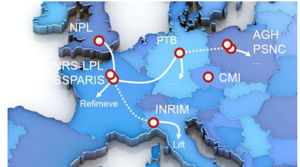
**A fiber network of about 6000 km in EU enabling bi-directional, coherent, optical frequency transfer**
