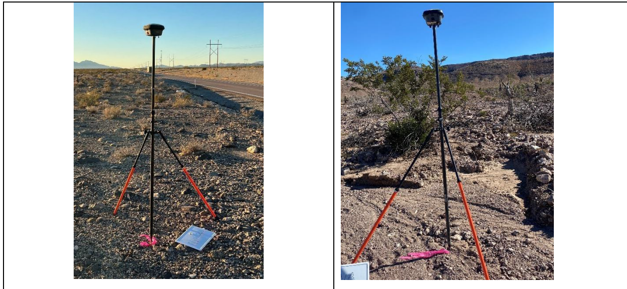
Figure IV.C.2 Locations that are not appropriate for GCPs and checkpoints.
