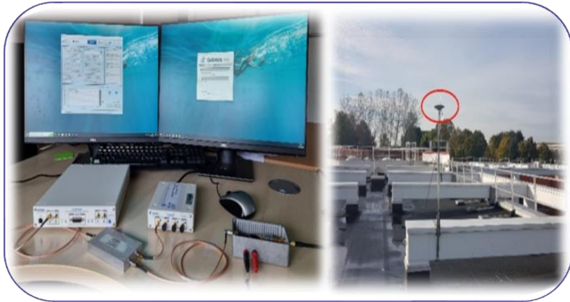
GNSS Signal Recording System and MATLAB-based Jammer connected to an antenna mounted on the roof of the building.
